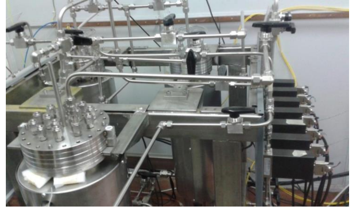
Membrane system for producing ultra-pure hydrogen via reforming of methane and olive mill wastewater
