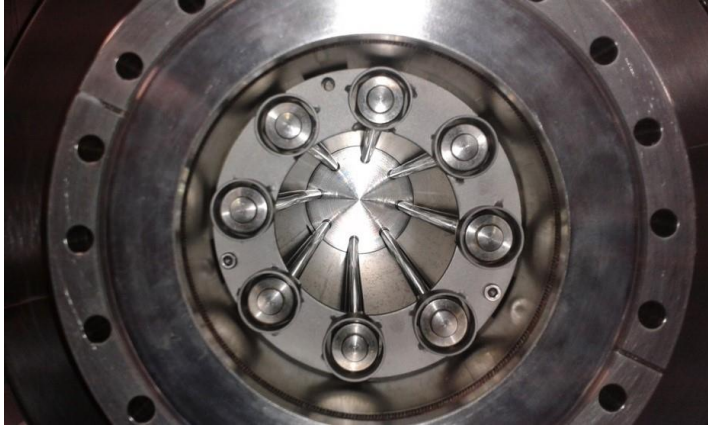
Internal view of the multi-tube membrane reactor built by ENEA for Eurofusion
