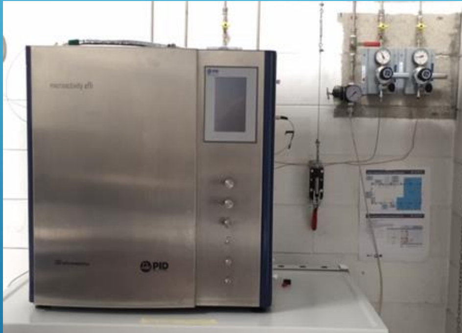
Reactor system for thermo-catalytic tests
