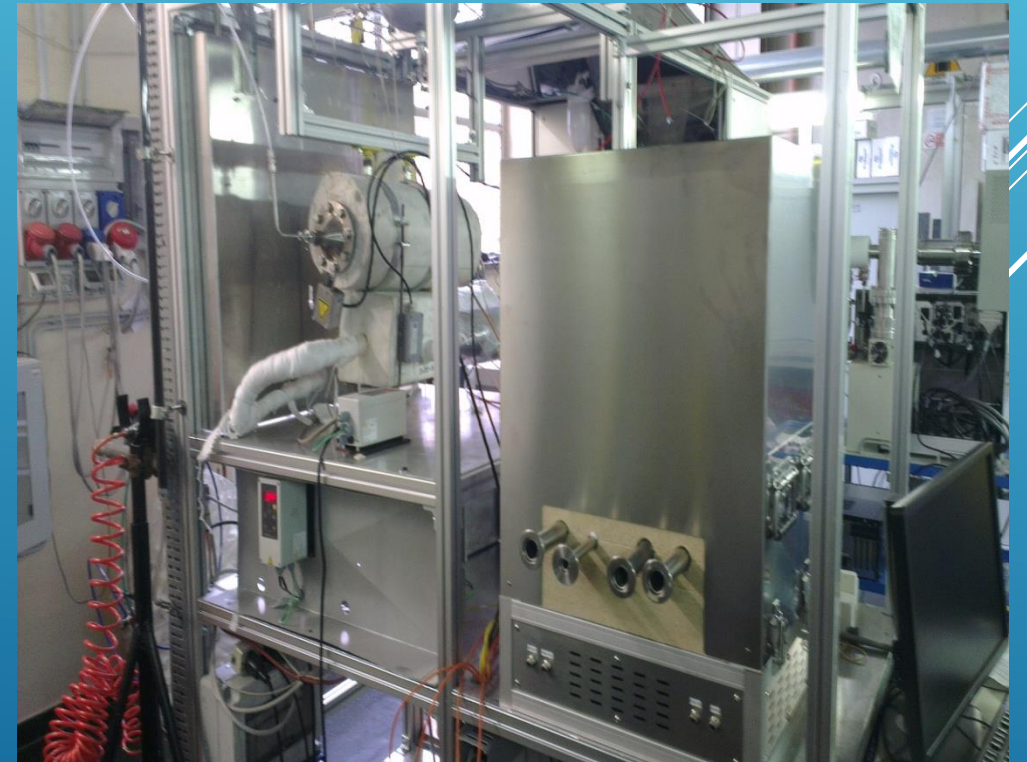
SOFC stack test bench
