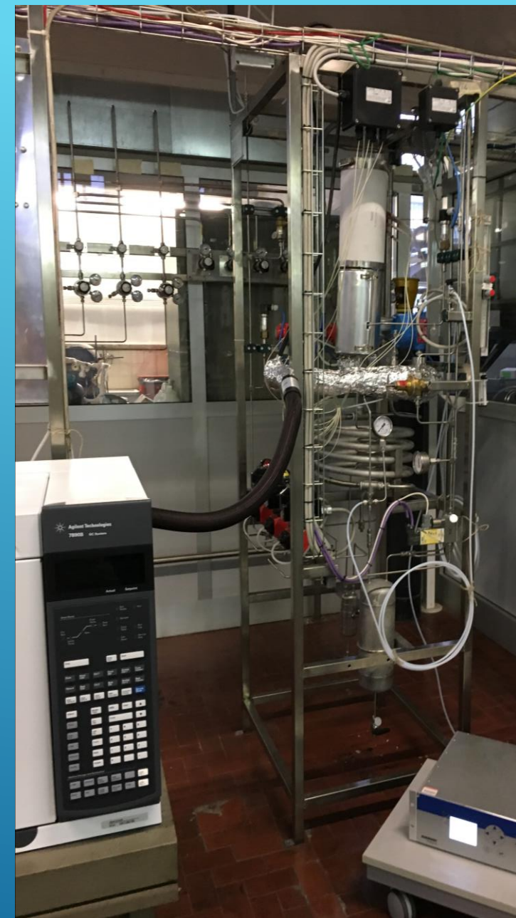
Production of synthetic chemicals through CO 2 hydrogenation tests
