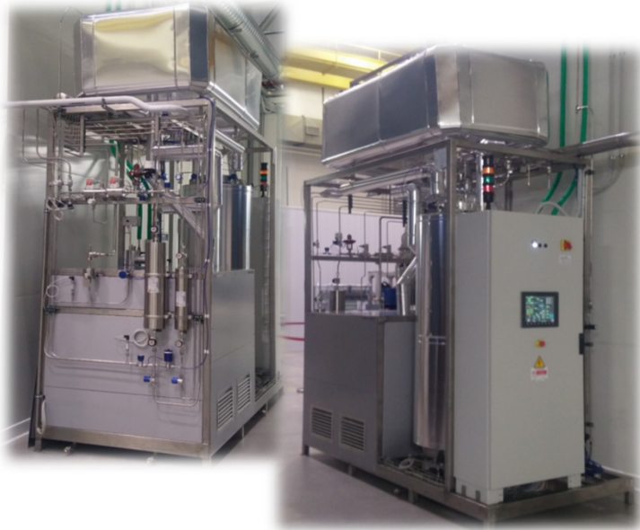
CO2 purification for snow cleaning process for Exomars space mission
