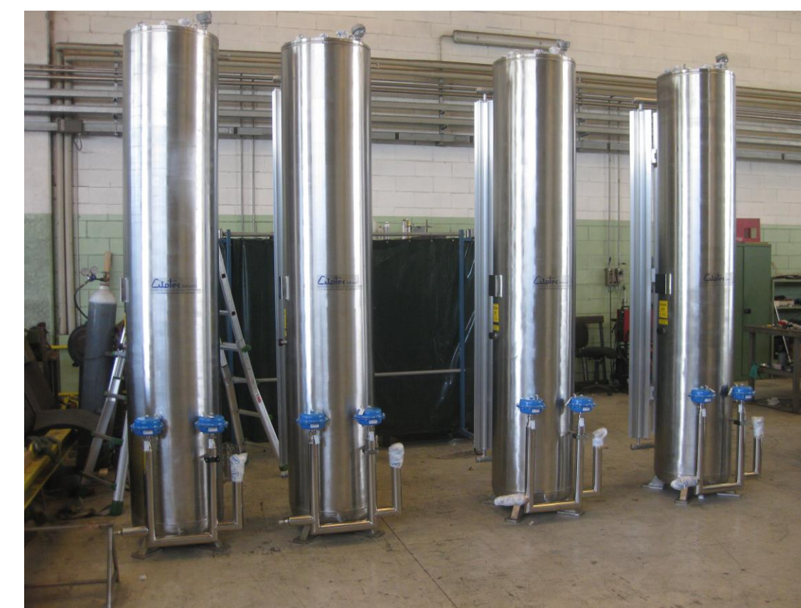
Hydrogen cryogenic purification units (up to 6.5 purity level)
